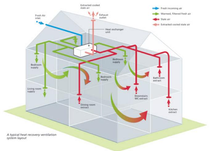
A typical heat recovery ventilation system layout
